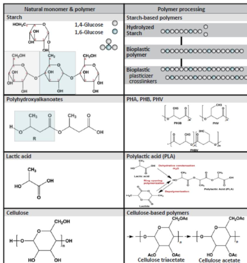
**Figure 7.** Important classes of currently developed bio-based plastics (adapted from Karan et al 2019)
