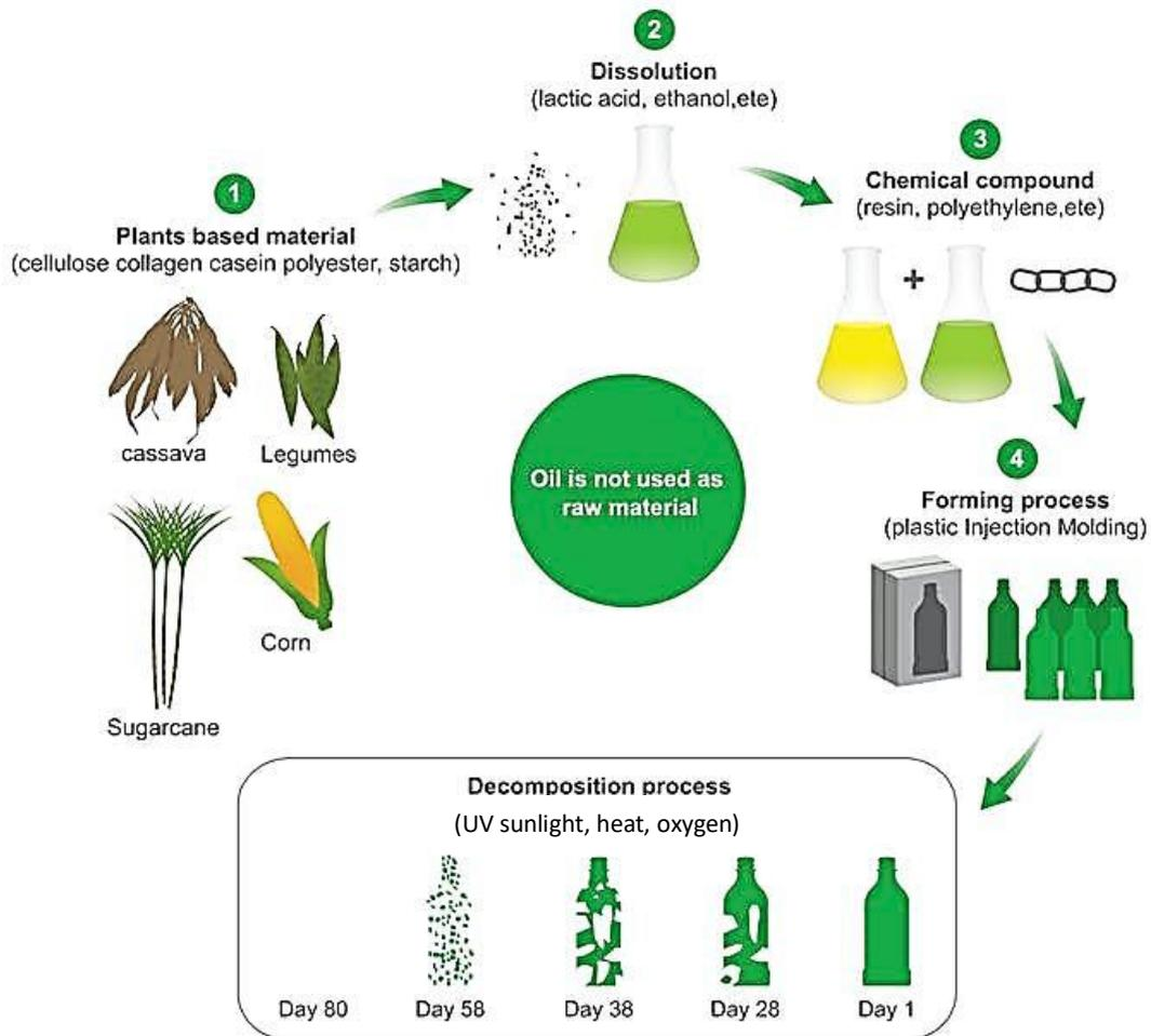
**Figure 4.** Life cycle of a bioplastic made of agricultural biomass through a chemical process. It is important to notice that not all bioplastics are biodegradable, only some of them are.
