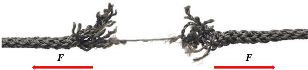
**Figure 3.** Schematic representation of tensile strength
